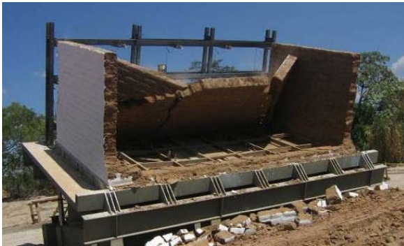
Tilting table test of Adobe house in El Salvador, JICA-TAISHIN Project
